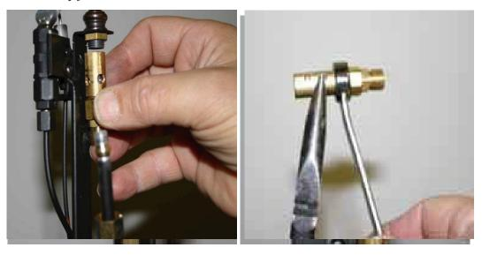
Use a small wire or a straight pin to clean out the tiny gas jets inside the burner orifice. Blow the soot out of the inside of the burner orifice. Reassemble the unit using pipe thread to avoid gas leaks.
